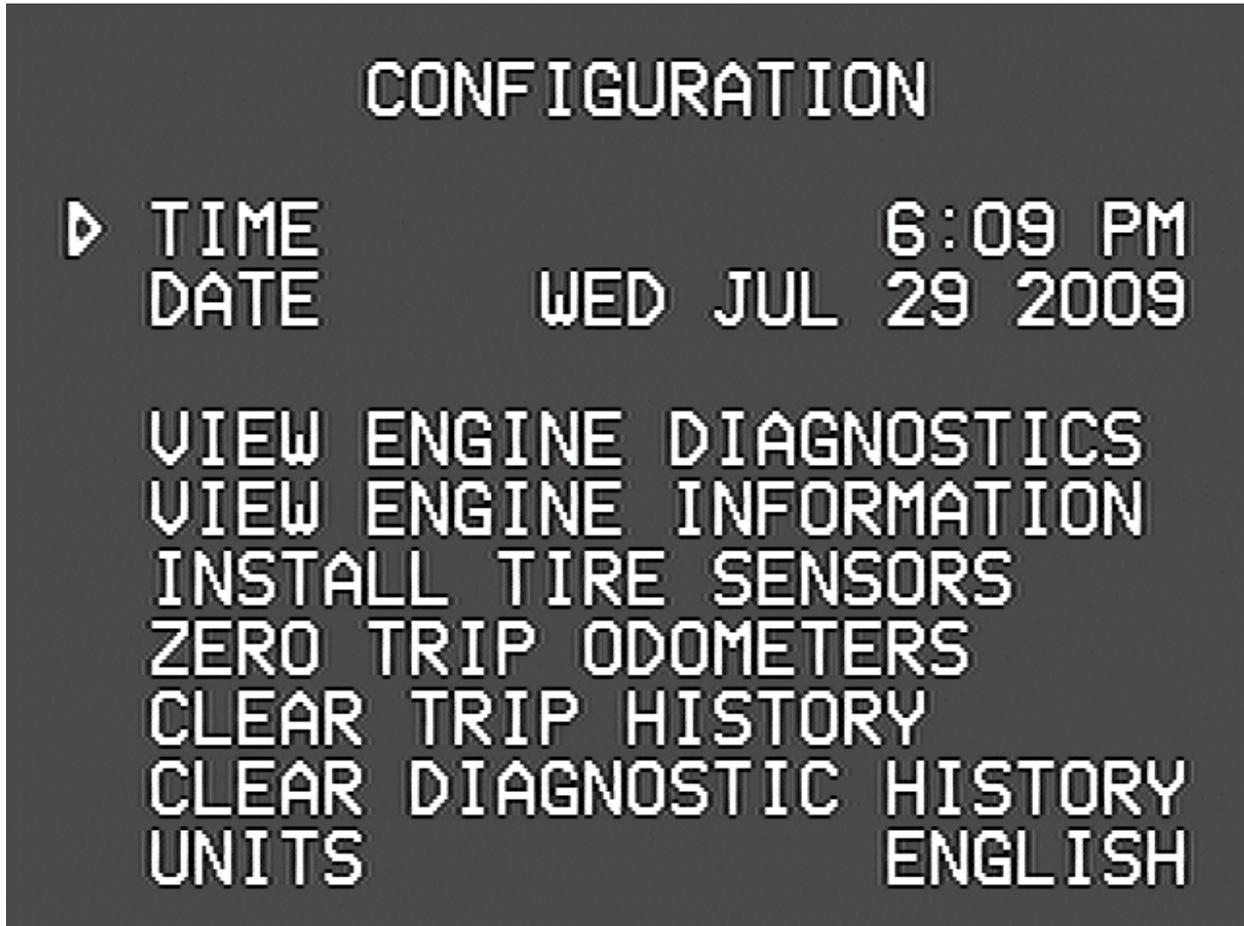
This screen appears with a second knob-press. It allows for adjusting the time and date, view engine diagnostics and other details, and access other features of the VMS 350.
