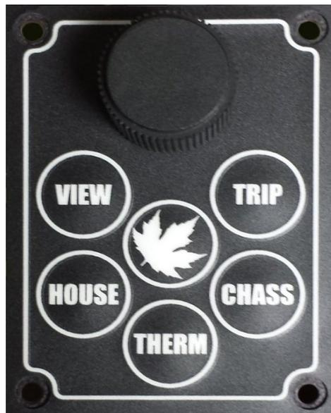
The keys all have specific functions as briefly shown here. Expanded details begin on page 8. While the VMS-350 is quite versatile, only the installed options will be accessible, based on your units' configuration.\*
