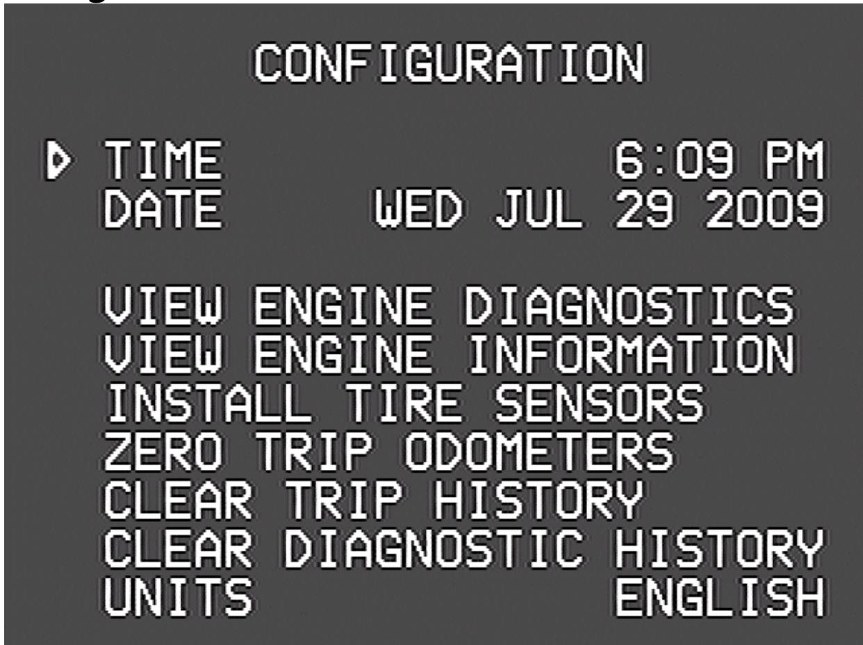
This screen allows you to adjust the time and date, view engine diagnostics and other details, and access other features of the VMS 350.
