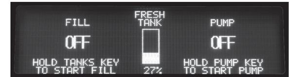
Note that the pump can also be controlled by switches mounted elsewhere in the coach. Those switches are tied to the Total Coach System, and they have exactly the same effect as holding the PUMP key for about one second.
