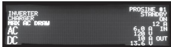
Holding the 120V key for a second will turn the Inverter on or off. Holding the INV key for a second will do the same for the charger. The only reason to turn either unit off is to reduce the small battery drain. The inverter in particular should be turned off if the coach is being placed in storage or is being left for several days. The charger should generally be left on.
